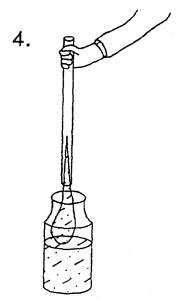
Place open tube sampler over appropriate sample bottle and remove gloved thumb.
