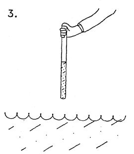
Remove open tube (thief) sampler from containerized liquid.
