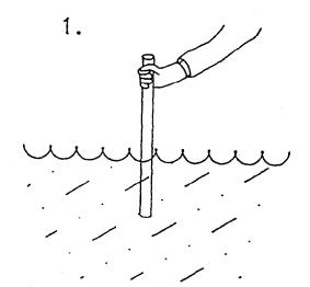
Insert open tube (thief) sampler in containerized liquid.
