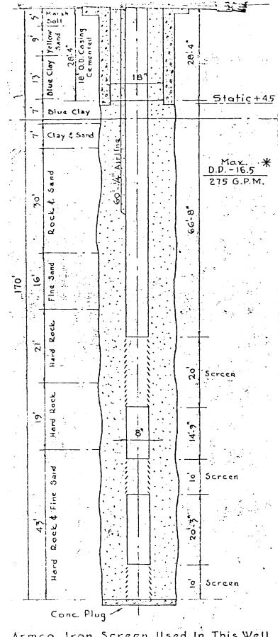
Armco Iron Screen Used In This Well
