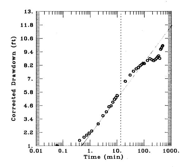
DATA SET: a: tw.dat 12/30/92 AQUIFER TYPE: Unconfined SOLUTION METHOD: Croper-Jacob ESTIMATED PAHAMETER: T = 0.04166  $ft^2/min$ S = 0.5446 TEST DATA: a = 0.255  $ft^3/min$  $r = 0.255 ft^3/min$
