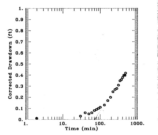
JATA SET: a: mw3.dat 01/05/93 AQUIFER TYPE: . Unconfined SOLUTION METHOD: Gooper-Jacob ESTIMATED PAHAMETERS: S = 0.06199 TEST DATA: u → 0.755 ft<sup>3</sup>/min 26. ft ţ. 52 b = 30. ft
