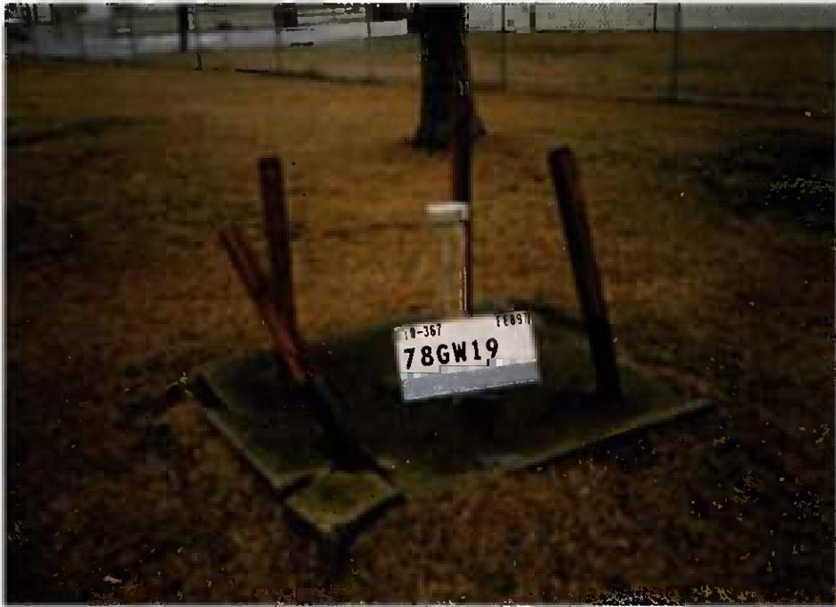
**Figure 4-11** Shallow monitoring well 78-GW19 was struck by a vehicle during hurricane debris removal activities.
