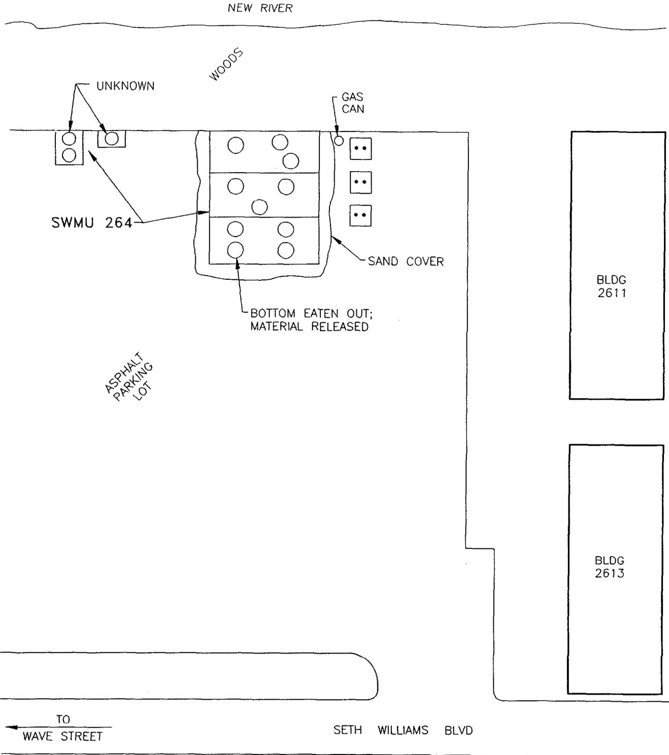
NOTE: DURING THE OCTOBER 1996 VISIT, THE ENTIRE PARKING LOT AT SWMU 264 WAS COVERED WITH WOOD CHIPS AND NO DETAILS WERE VISIBLE. THE DETAILS IN THIS DRAWING WERE NOTED BY ENSAFE, INC. IN NOVEMBER 1993.
