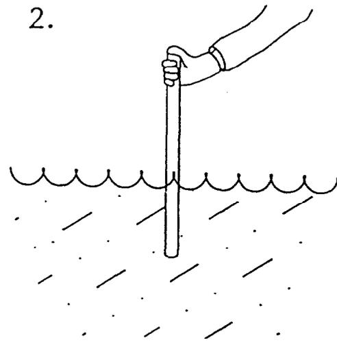
Cover top of sampler with gloved thumb.
