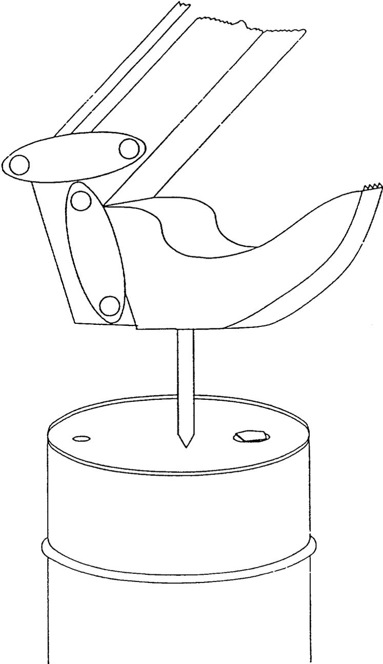
Figure 5: Hydraulic Drum Opener
