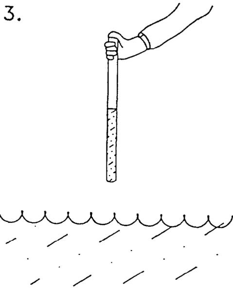
Remove open tube (thief) sampler from containerized liquid.
