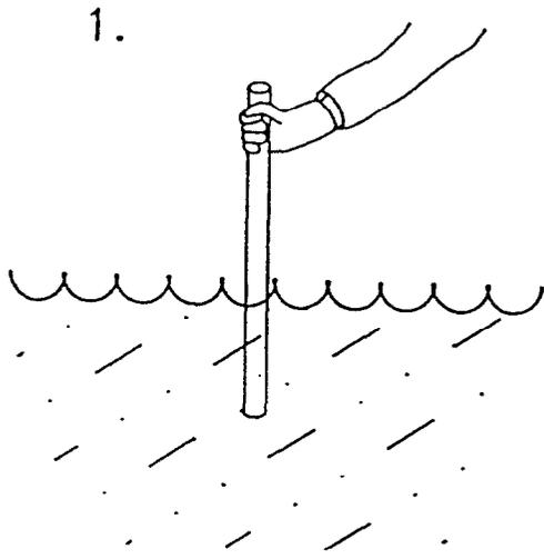
Insert open tube (thief) sampler in containerized liquid.
