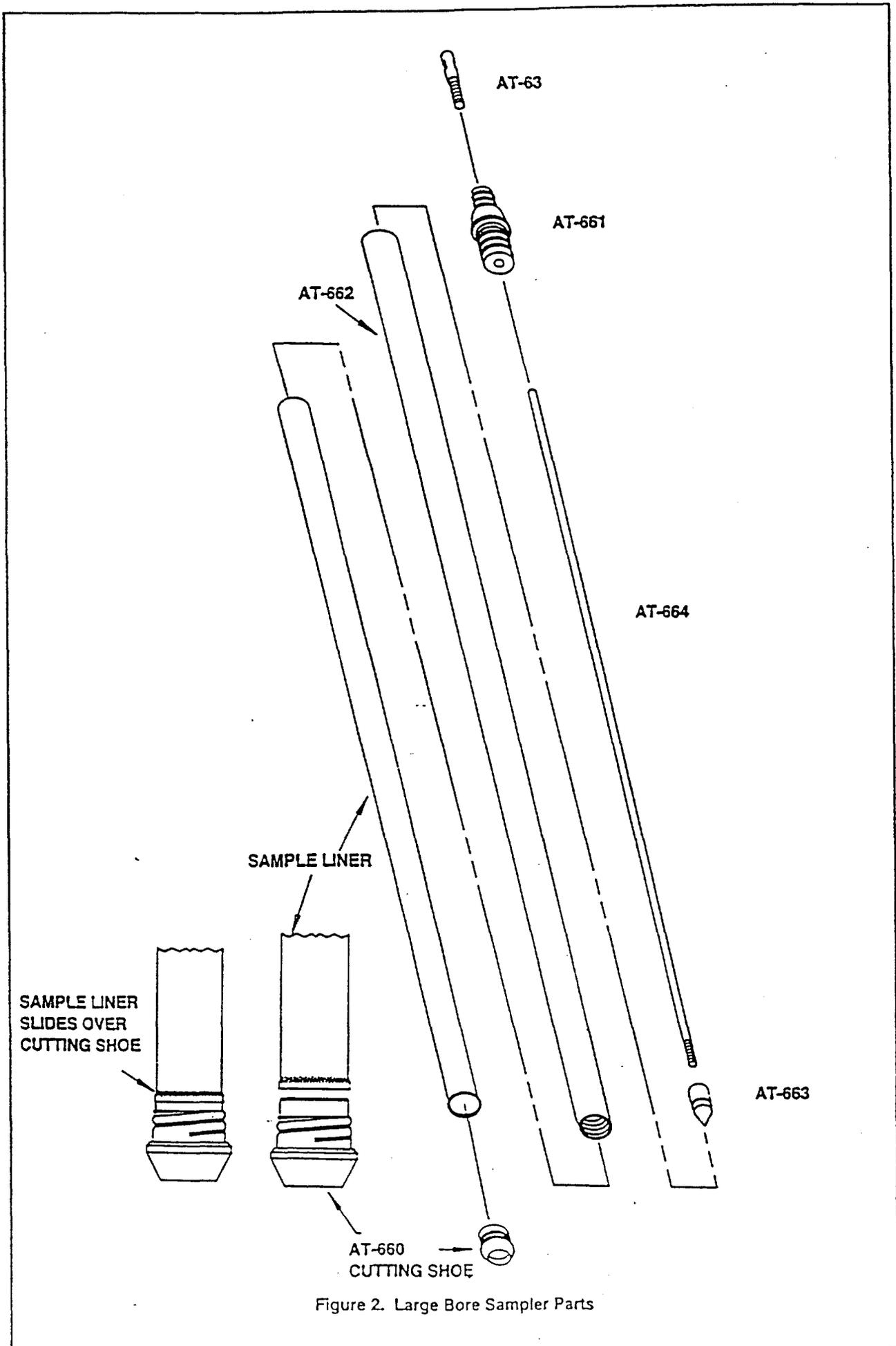
Figure 2. Large Bore Sampler Parts
