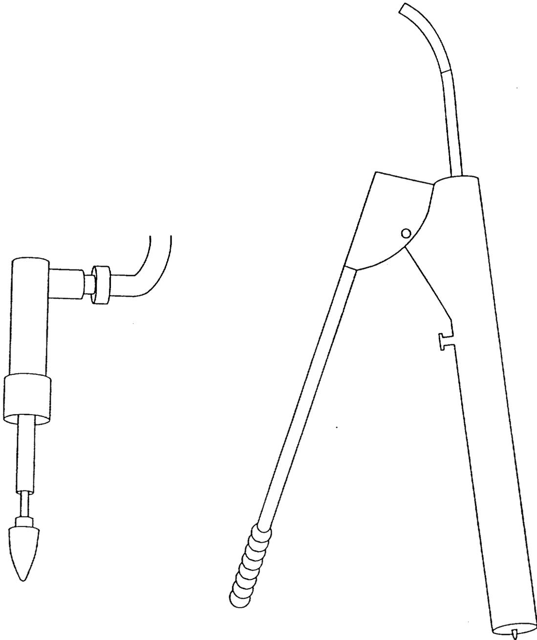
Figure 6: Pneumatic Bung Remover
