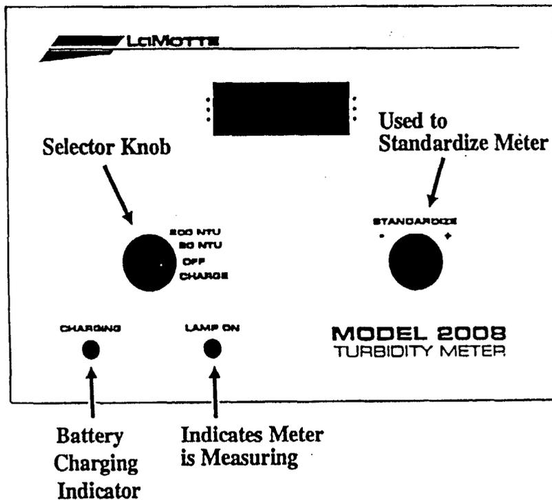
The Model 2008 portable turbidimeter is acceptable for turbidity measurements reportable under either the National Primary Drinking Water Regulations (NPDWR) or the EPA's Surface Water Treatment compliance monitoring program. This instrument is suitable for testing municipal waters, food and beverage processing waters, and any aqueous solutions in which control of clarity is critical. The unit may be operated from line power via an AC adapter or from self-contained rechargeable batteries.
