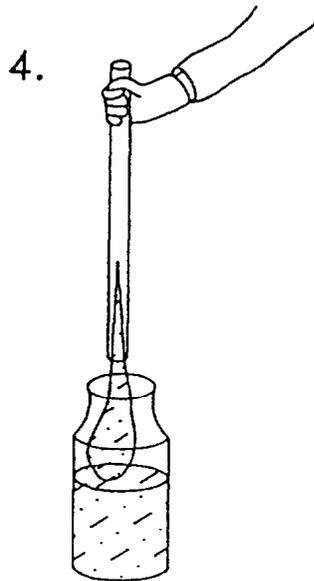
Place open tube sampler over appropriate sample bottle and remove gloved thumb.
