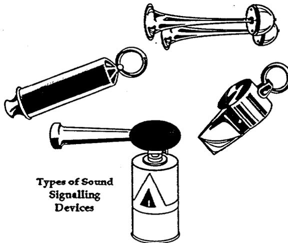
Types of Sound Signalling Devices
