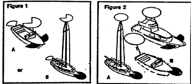
Power-driven vessels of less than 20 meters, shall exhibit navigation lights as shown in Figure 1. Vessels of less than 12 meters in length, may show the lights in either Figure 1 or Figure 2.
