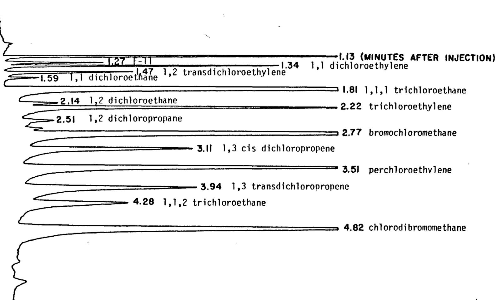
Figure 1 - Chromatogram showing the analysis of selected volatile contaminants in water by direct injection on to capillary column (oven temp. 50°C isothermal). Analyses of soil gas or water are identical by TRC method and require 5 minutes or less to perform.
