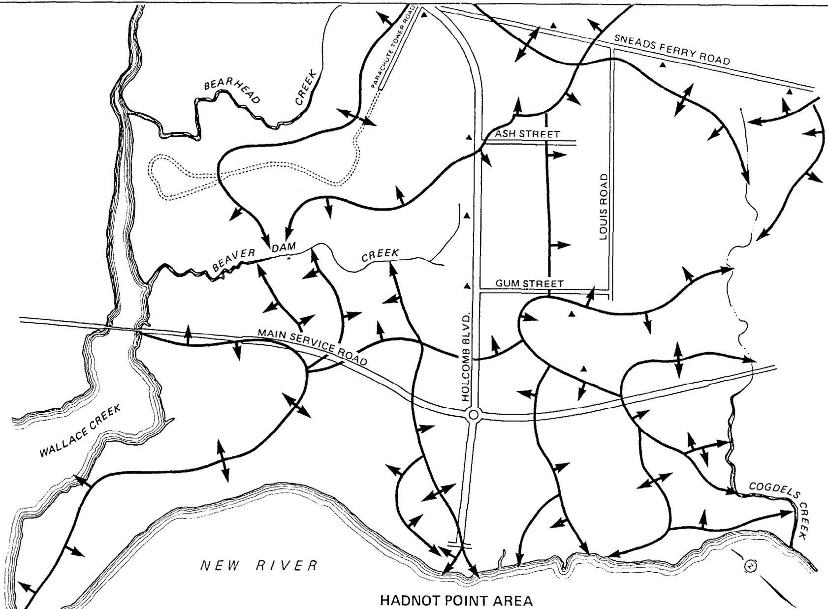
FIGURE 5-2. Surface Water Drainage Sub-Basins at Hadnot Point, MCB Camp Lejeune
