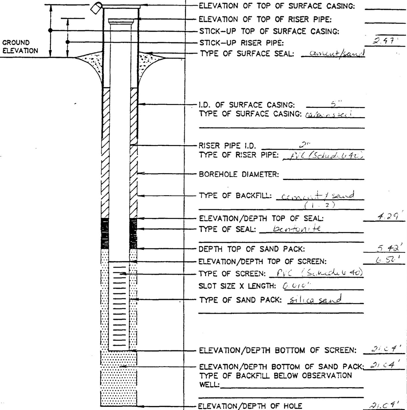
ELEVATION OF TOP OF SURFACE CASING: \_\_\_\_\_
