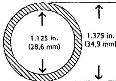
Actual size of Large Bore Sample Tube. The Large Bore Sampler gives an ample I.D. for core recovery while maintaining a small O.D. for ease of driving.
