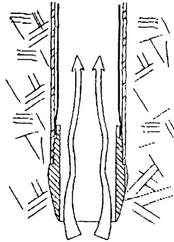
Geoprobe soil samplers feature liners that fit over the end of the cutting shoe. This feature, which was pioneered by Geoprobe, allows soil to flow into the liner without lodging behind the liner.
