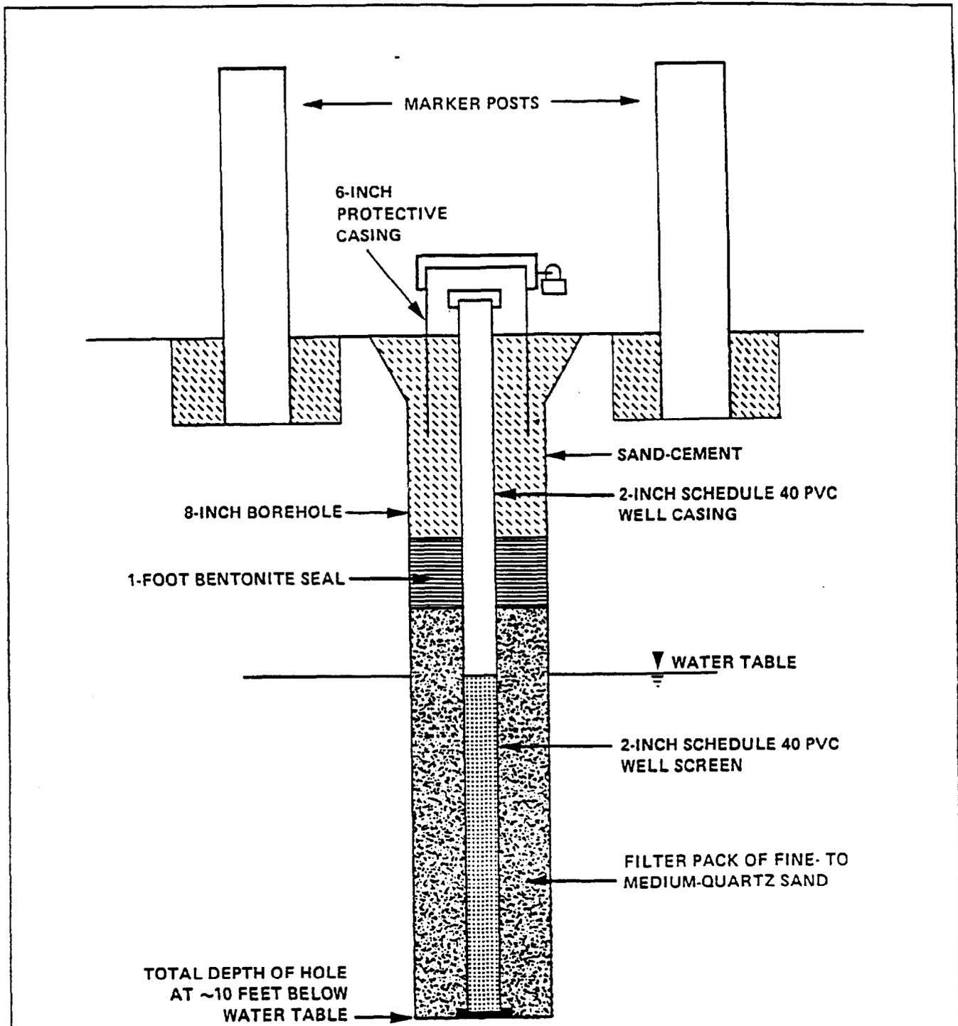
FIGURE A-1. Recommended Monitoring-Well Construction
