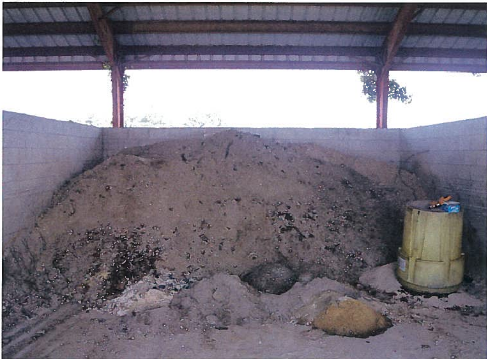
Photo 2; Soil stockpile comprised of oil/water separator grit chamber solid waste and used oil dry.
