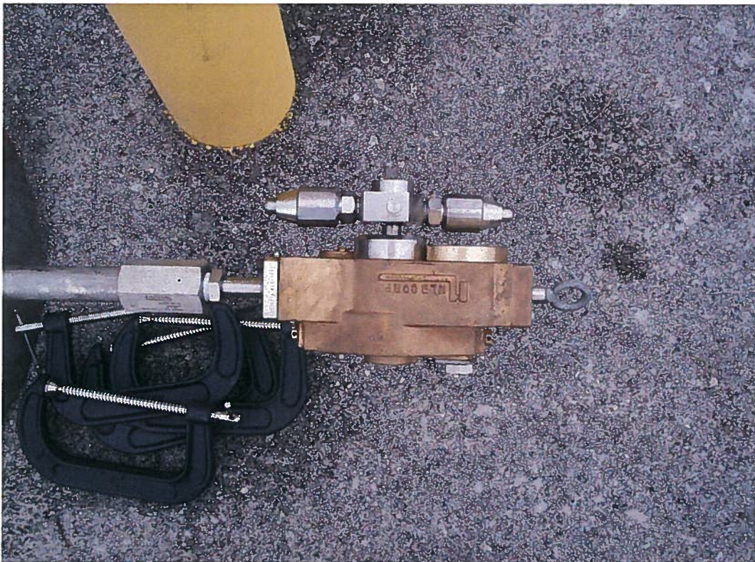
Photo 7: Hydro blaster rotating head and spray nozzle assembly.
