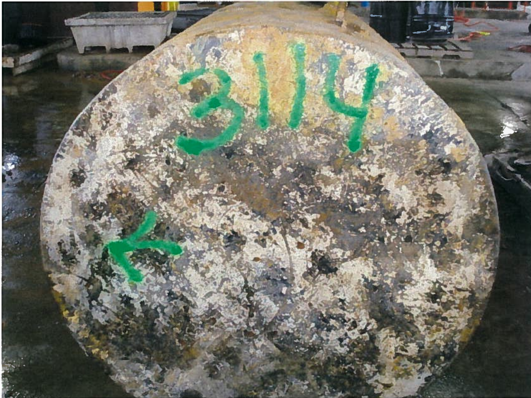
UST TT-3114 after cleaning at RCRS, Building 977
