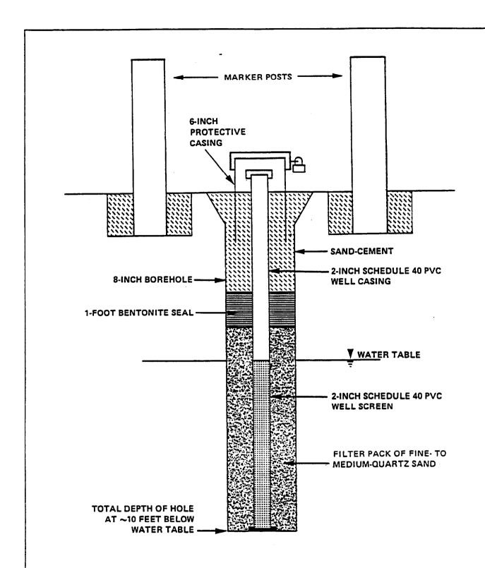
FIGURE A-1. Recommended Monitoring-Well Construction
